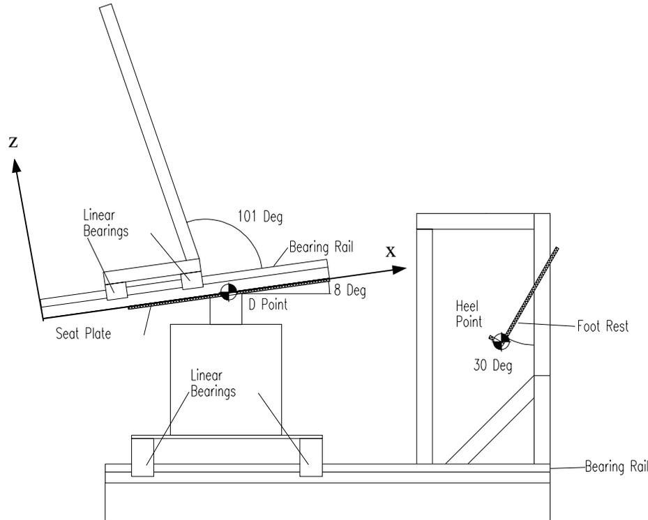
**Figure 5. Simulated drive posture measurement station.**
