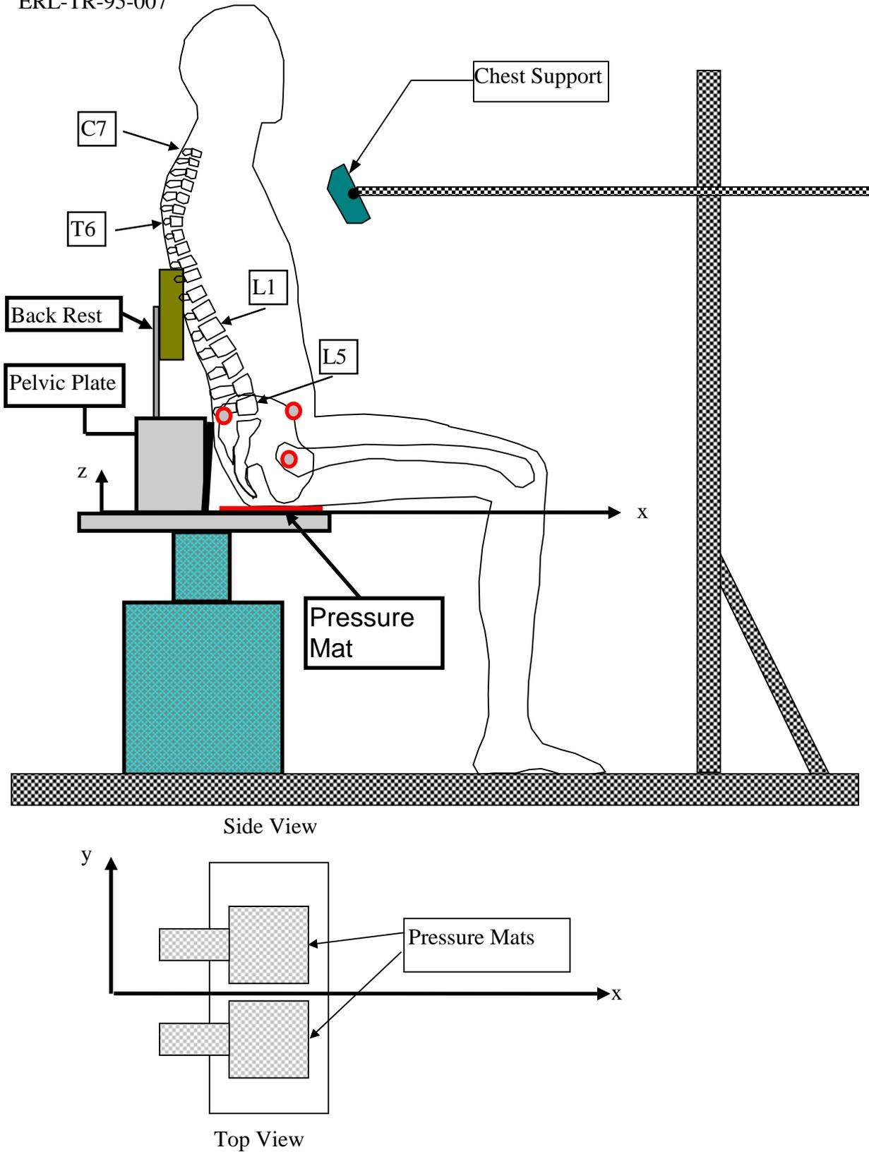
**Figure 2. Position of the subject, location of pressure mats and illustration of the landmarks measured for this research.**
